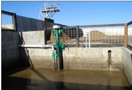
EQIP cost-share could have been used to help fund at least four of the practices shown here (pit, pump, separator, drystack).
