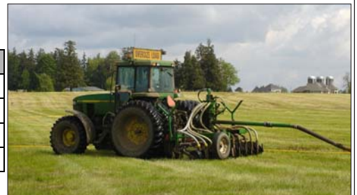
Manure Injection is an application method that makes the best use of ammonia in manure, while minimizing ammonia loss to the air.
